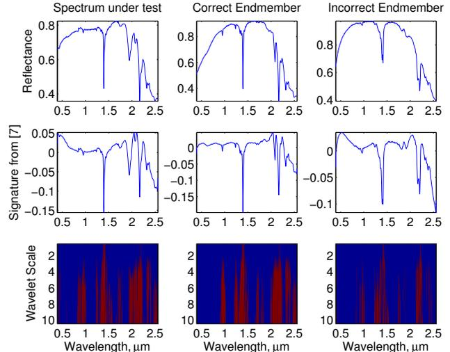
**Fig. 3:** Comparison of classification results for USGS spectral library. Left column: spectrum being identified (*pyrophy3*); middle column: correct endmember (*pyrophy2*); right column: incorrect endmember returned by the approach of [7] (*kaolini1*). Top row: reflectances; middle row: filtered signatures from [7]; bottom row: labels from NHMC for wavelet coefficients.
