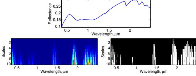
**Fig. 1:** Top: Example spectral signature ( $N = 325$  samples). Left: Corresponding CWT coefficient array ( $s = 9$ ) using a Daubechies-4 wavelet. Small/large coefficient magnitudes are shown in blue/red. Right: State labels obtained for the example spectral signature using a NHMC model. White corresponds to large labels; black to small.
